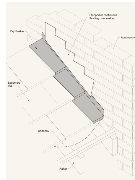
Edgemere abutment with dry fix soakers
